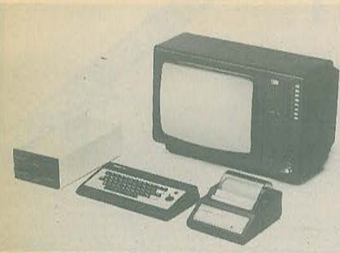
de COMX 35 - Keyboard - Thermoprinter - dubbele floppy-drive
